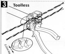
Insert the wires through the cap and seat the wires in the correct slots according to T568A or T568B. Trim the wires flush with the cap. It's recommended the tip of wires is not more than 0.2mm.
