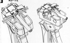
Use KJ-TL series to terminate and cut 4-pairs of wires simultaneously finishing installations.
