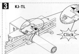
Insert the wires through the cap and seat the wires in the correct slots according to T568A or T568B. Match with the black triangle and align the cap with IDC until it clicked as shown.
