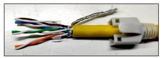
4. Insert each pair of cables into the 4 grooves of guide C (do not undo the twisting) (orange pairs and brown pairs in 2 of the grooves on the left and right) green pairs and blue pairs in the top and bottom 2 grooves)
