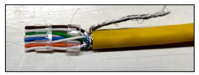
5. Insert the wires into cable guide B according to the T568B or T568A assignment.
