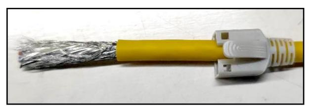
2. Feed the cable through sleeve D and strip approx. 30 mm of the outer sheath of the raw cable.
