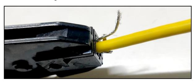
8. Crimp connector A with the crimping pliers.
