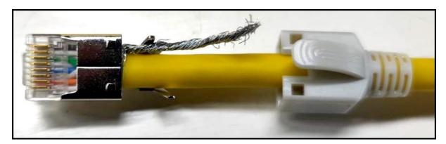
7. Insert the cable with both guides B and C into connector A.
