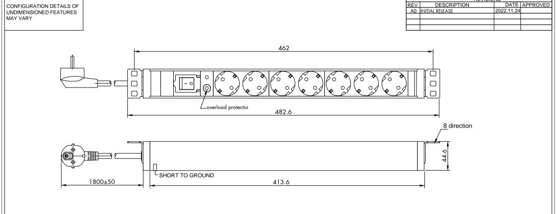
NOTE: RATING VOLTAGE:250VAC 50/60HZ RATING CURRENT:16A MAX. CURRENT:16A MAX. POWER:4000W
