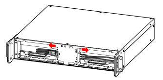
Step 4 Pull out the left and right battery pack.
