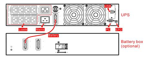
Figure3-3 Wiring diagram of IST3-J 2kVA/IST3-J 3kVA
