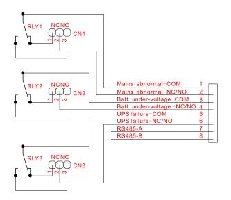
Figure2-17 Pin definition of RS485 and dry contact
