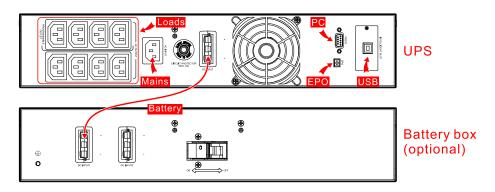
Figure3-2 Wiring diagram of IST3-J 1kVA
