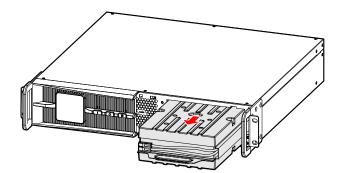
Step 5 Push the new battery pack into UPS.
