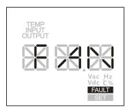
Figure2-25 Fan fault
