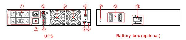
Figure2-7 Rear panel of IST3-J 2kVA / IST3-J 3kVA
