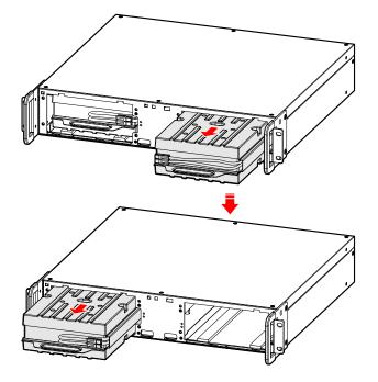
Step 5 Push the left and right new battery pack into battery box.
