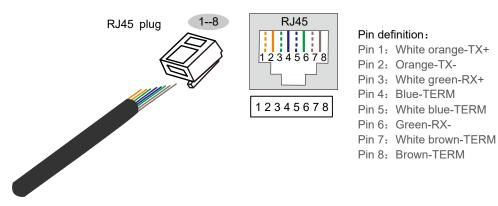
Figure2-20 The pin definition of the NETWORK port
