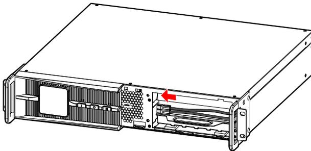
Step 7 Install the battery plate.
