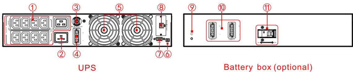
Figure2-7 Rear panel of IST3-J 2kVA / IST3-J 3kVA
