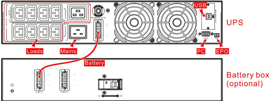
Figure3-3 Wiring diagram of IST3-J 2kVA/IST3-J 3kVA
