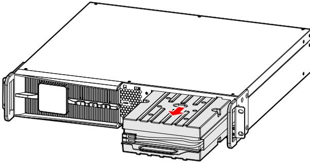
Step 5 Push the new battery pack into UPS.
