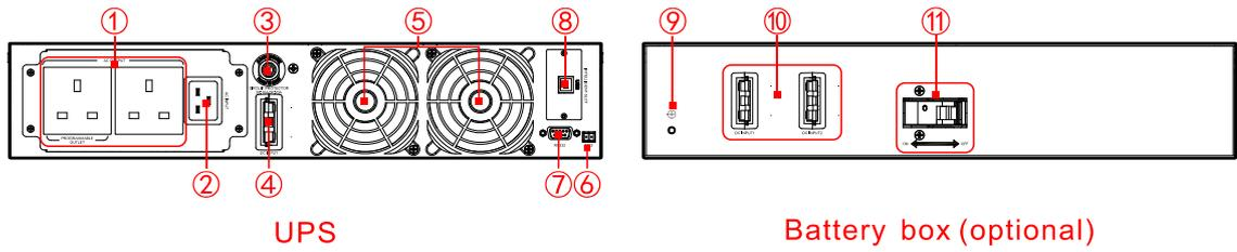
Figure2-13 Rear panel of IST3-J 2kVA / IST3-J 3kVA
