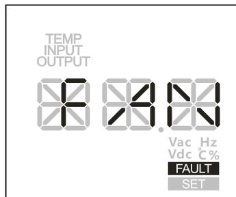
Figure2-25 Fan fault
