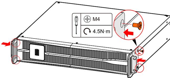
Step 3 Fix battery box (optional) on the rack.
