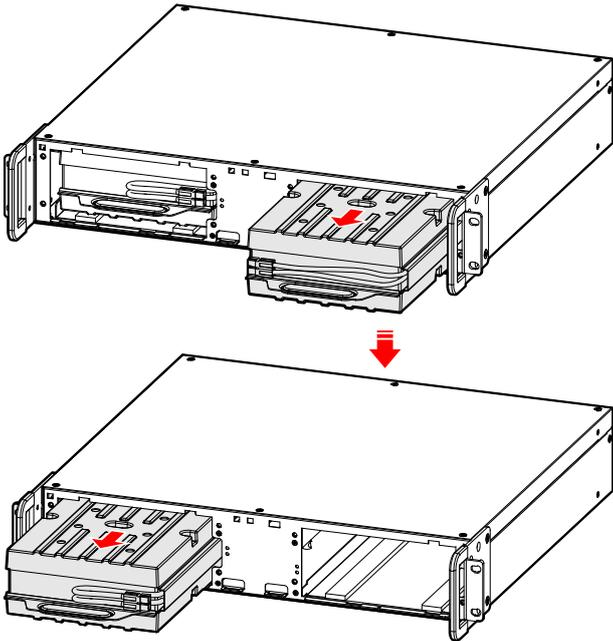
Step 5 Push the left and right new battery pack into battery box.
