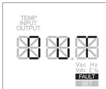
Figure2-26 Output fault
