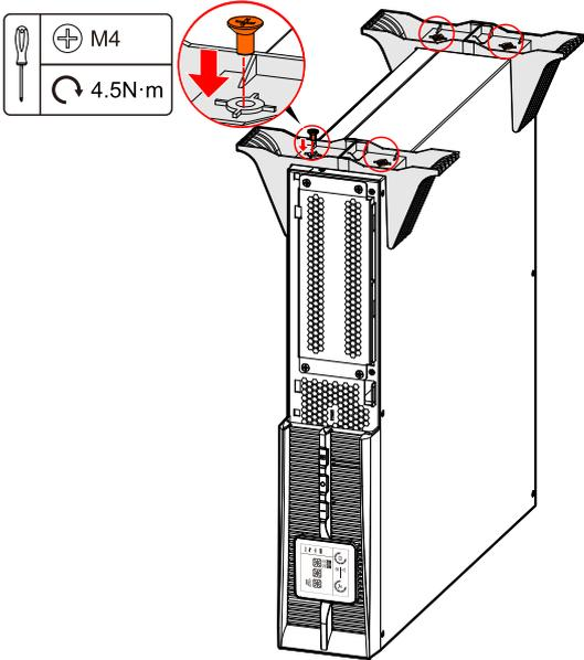
Step 4 Place UPS with support bases, and then install the plastic panel.
