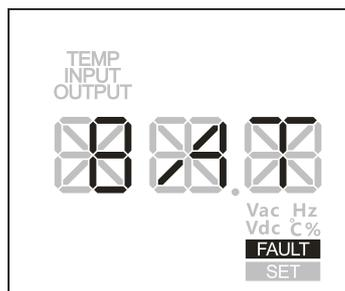
Figure2-27 Battery fault
