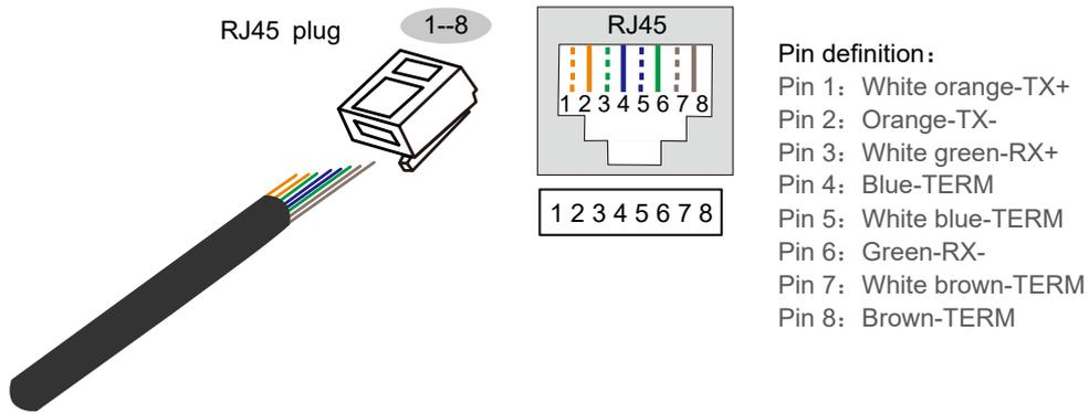
Figure2-20 The pin definition of the NETWORK port
