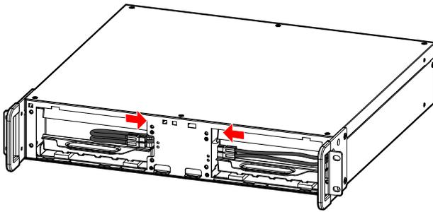
Step 7 Install the battery plate.
