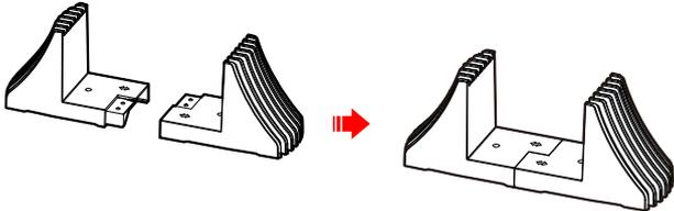
Step 3 Fix the support bases on UPS.
