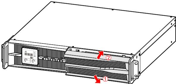
Step 9 Finish battery pack installation.
