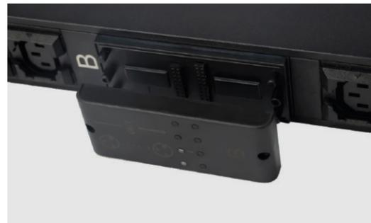
Monitoring the power metrics of 8 outlets and control their on/off switching
