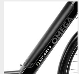
36V 10.4Ah 374Wh battery, integrated into the frame
