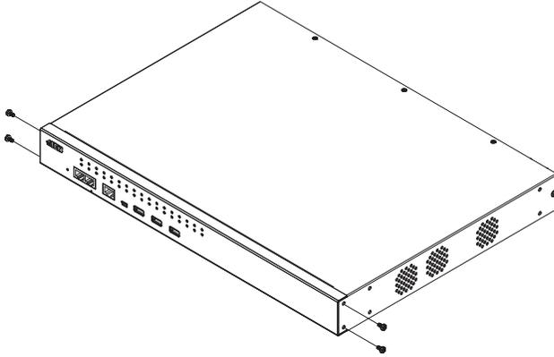
2. Use the M3 x 8 Phillips head hex screws supplied with the rack mount kit to screw the rack mounting brackets into the front of the unit.
