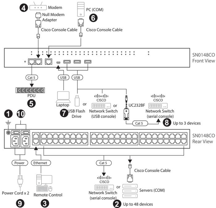
**Note:** A SN0148CO serial console server is used as an example to illustrate the installation. As for other serial console servers, the installation is identical with fewer serial ports.
