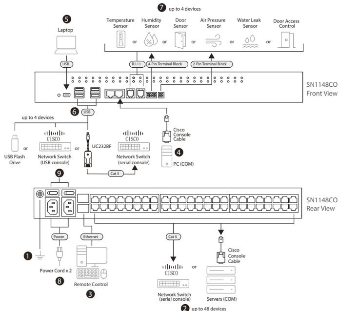
Note: A SN1148CO serial console server is used as an example to illustrate the installation. As for other serial console servers, the installation is identical with fewer serial ports.
