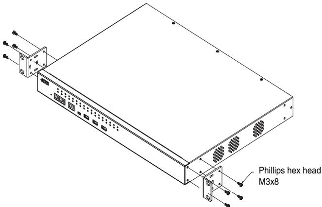
3. Position the device in the front of the rack and align the holes in the mounting brackets with the holes in the rack. Screw the mounting brackets to the rack.
