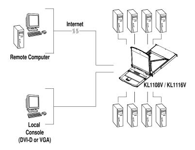
For added convenience, ports for an external keyboard, monitor (DVI-D or VGA), and mouse are provided on the rear panel — permitting you to manage the switch from a local console. There is also an external USB mouse port on the keyboard module, allowing you to use an external mouse, rather than the touchpad.
