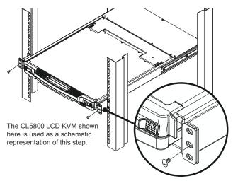
3. While the first person still holds the unit in place, the second person slides the left & right L-shaped brackets into the unit's side mount brackets from the rear, installing four screws in the brackets to secure them in place.
