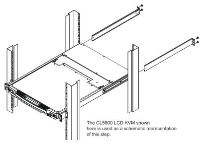
4. After the L-shaped brackets are secured, tighten all the screws.
