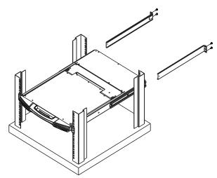
3. After the L-shaped brackets are secured, tighten all the screws.
