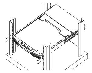
2. While the first person still holds the unit in place, the second person slides the left & right L-shaped brackets into the unit's side mount brackets from the rear, installing four screws in the brackets to secure them in place.
