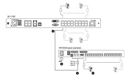
**Note:** The diagram above shows an installation with the KL1116V. Cascading the KL1108V is same as the KL1116V and only differs in that it provides fewer KVM ports.
