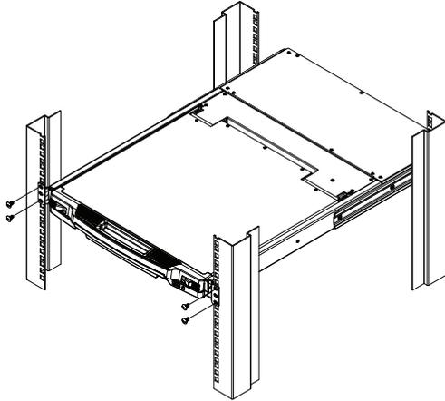
2. While the first person still holds the unit in place, the second person slides the left & right L-shaped brackets into the unit's side mounting brackets from the rear, installing four screws in the brackets to secure them in place.
