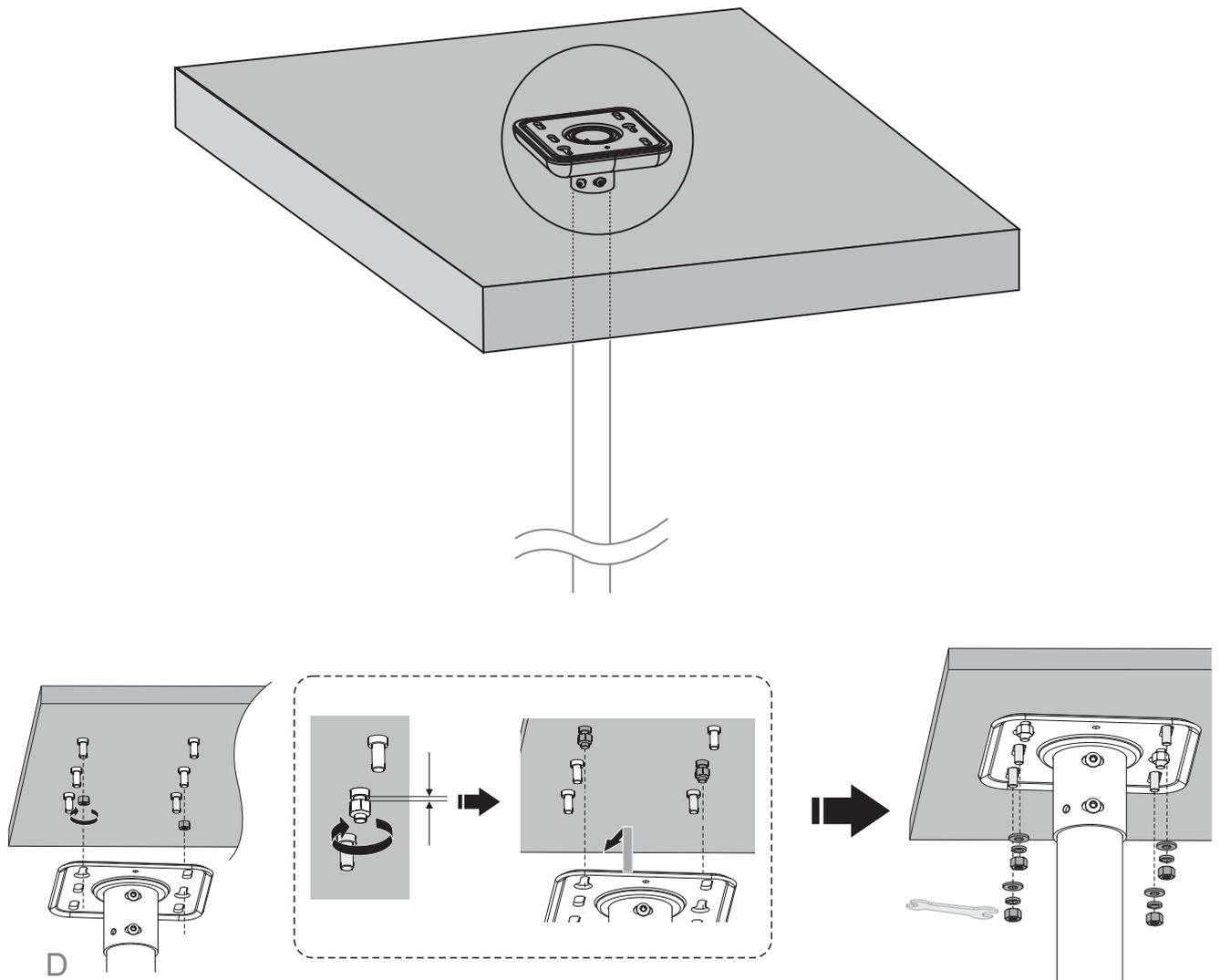
**8 Abdeckungen anbringen (Boden / Decke) | Attach the cover (Floor / Ceiling)**
