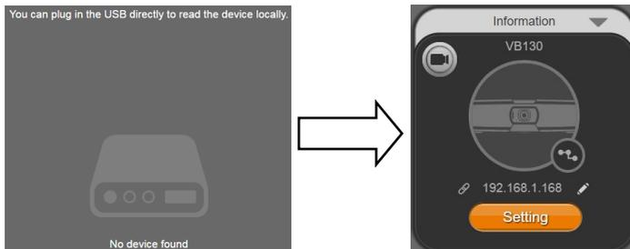
5. Set up IP address. The camera default IP address is 192.168.1.168. Click pencil icon (✎) to edit IP address.
