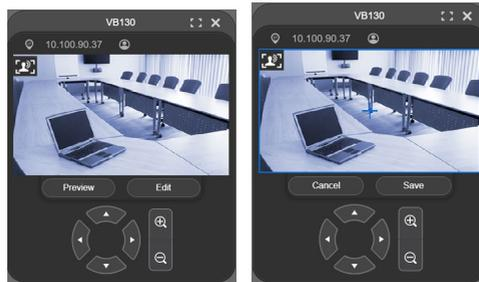
You can also use remote control by pressing **(P)** and then **(2)** to save presentation area. After adjusting the desired image proportion and position, press **(P)** then **(2)** to confirm the presentation area. Please notice that this area is beyond 0~9 preset points on remote control.
