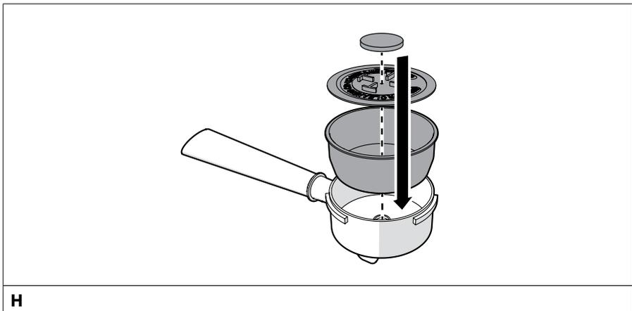
2. Place the **double cup filter** 19 into the **portafilter** 21.
