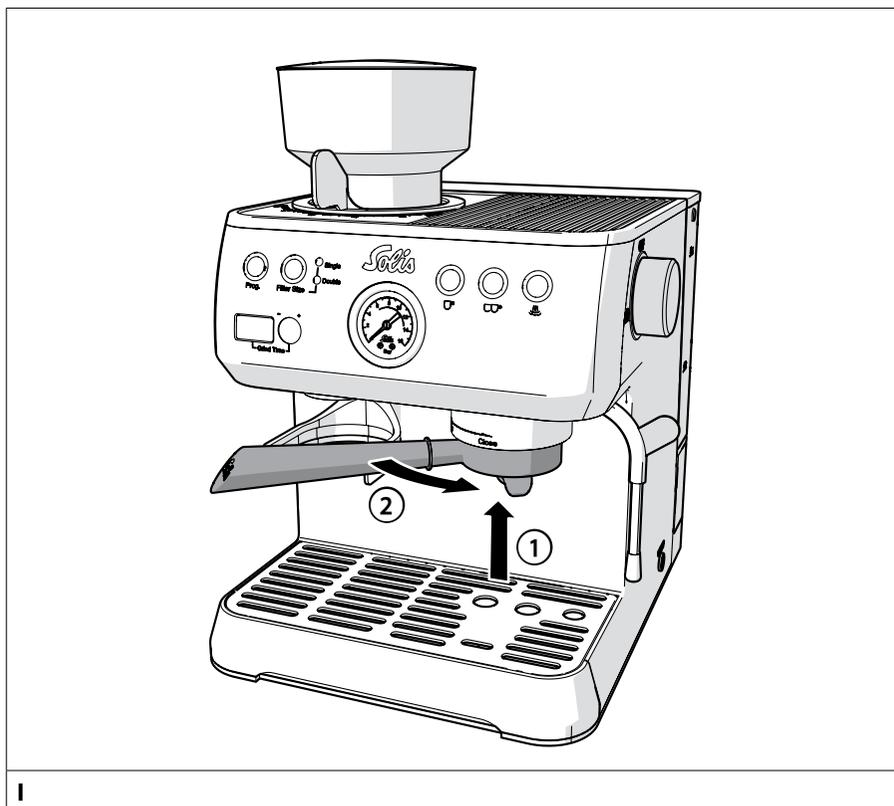
4. Insert and rotate the **portafilter 21** into the **brewing head 4** (see image I). Make sure the handle is aligned with the **CLOSE** marking.
