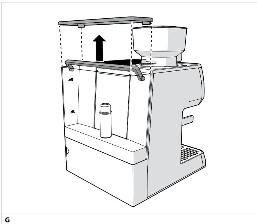
To replace the water filter cartridge:
